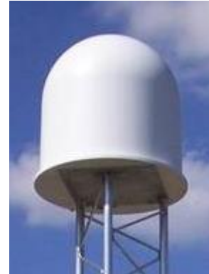
Figure 1. This is the MDR on a Rohn 45 G Tower.
