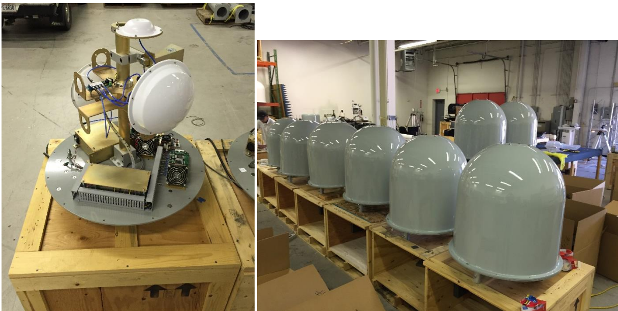
Figure 4. Left -- MDR with radome off. This model has two 7-degree beam antennas, one 360-degree antenna, and one 29-degree antenna. Right picture shows a shipment of MDR's going to protect oil refineries in the Middle East.
