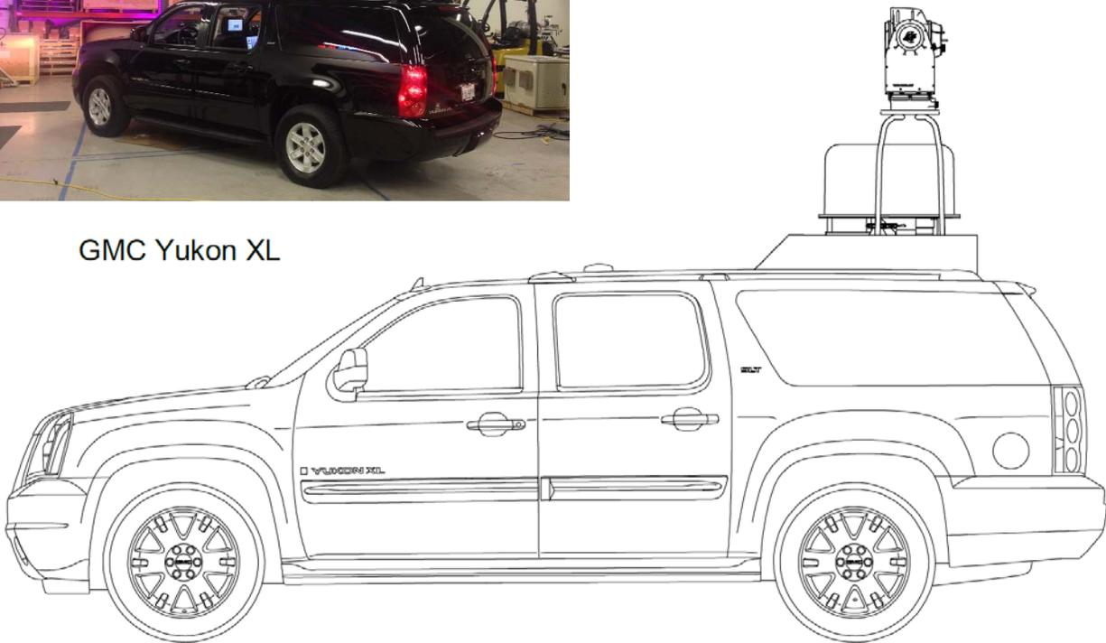
Figure 5. Optional Camera Mount shown here. This model allows for the camera the radar to be removed when not in use. It also allows a wider selection of cameras to be mounted on the vehicle.
