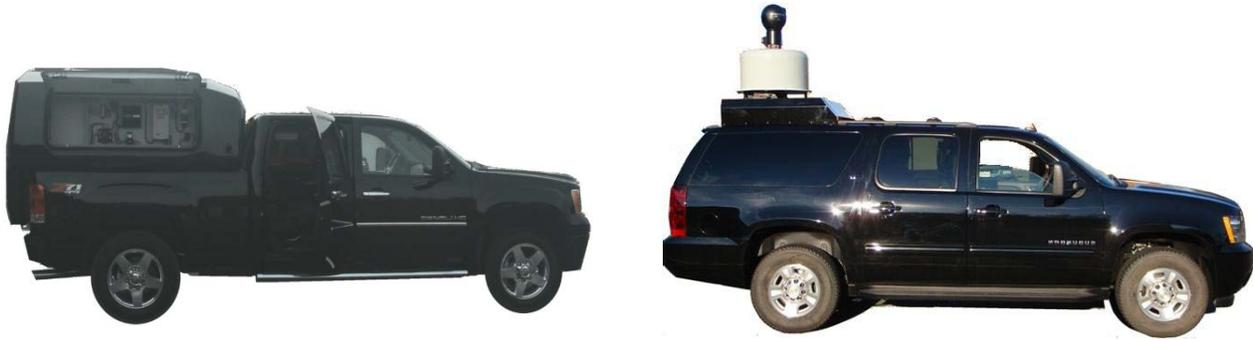
Figure 4. The two DMT MSV systems are shown here. The Sierra Truck System on the left and the Yukon (or Suburban) shown on the right.
