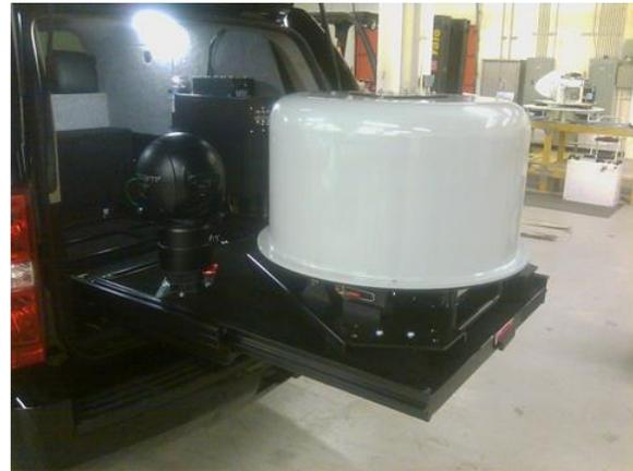
Figure 2. Pull-out tray for sensors when they are being prepared for long-range shipping.
