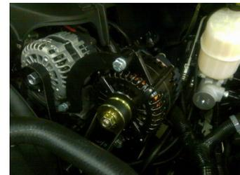
*Figure 1. DMT adds a second alternator to power sensors.*
