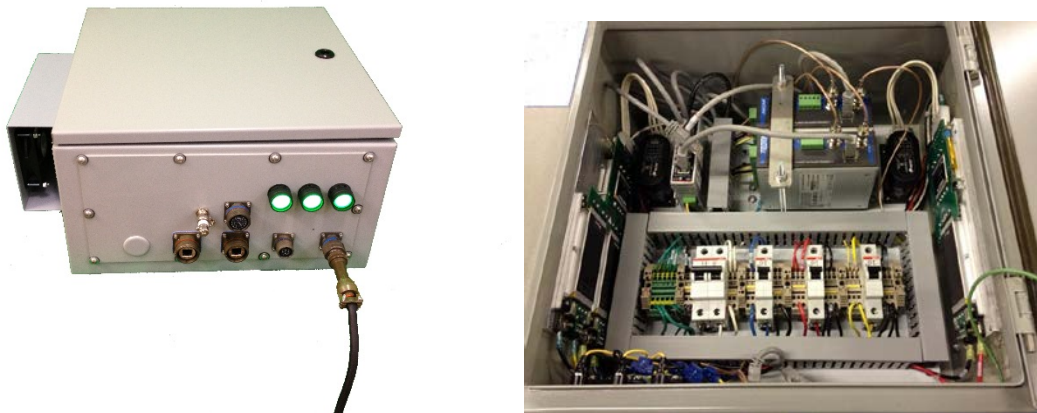
Figure 4. This is the DCPM with 1-port video server. Standard system is an Axis Q7424-R 4-port video server. Right picture shows hardware inside the enclosure. Circuit breakers inside the box protect inside and attached hardware.
